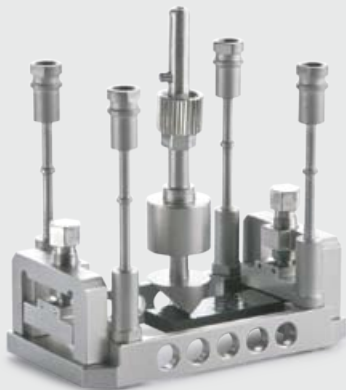
Special sample holder for bending of composites
