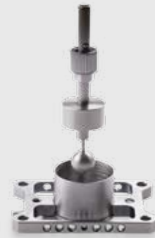
Special sample holder with ball-shaped pushrod for curing of low viscosity liquids
