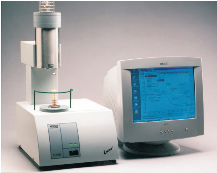
Figure 1: Simultaneous Thermal Analyzer STA 409 PC Luxx®
